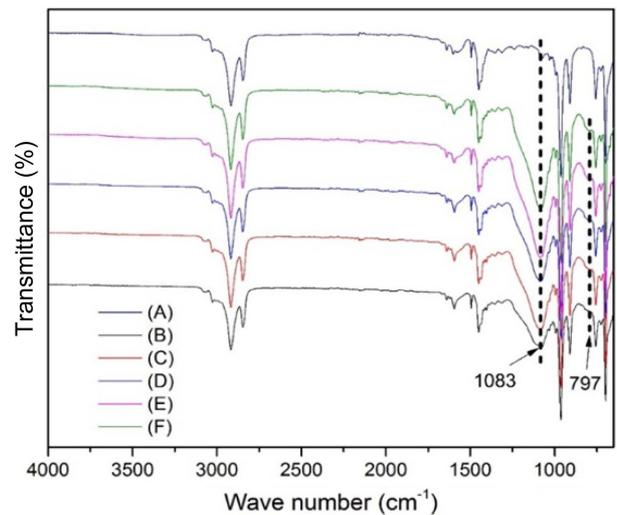
Figure 4. FT-IR spectra of neat SBR and silica-reinforced SBR.
