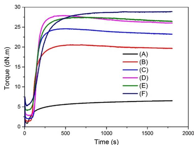
**Figure 6.** Torque versus time traces for different contents of TEOS.
