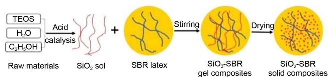
**Figure 1.** The process of preparation of silica-reinforced SBR.
