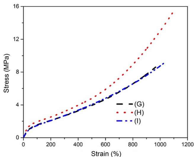
**Figure 11.** Tensile strength test of silane coupling agents (G: with TESPT; H: with GPTS and I: with ETS) modified silica in SBR matrix.
