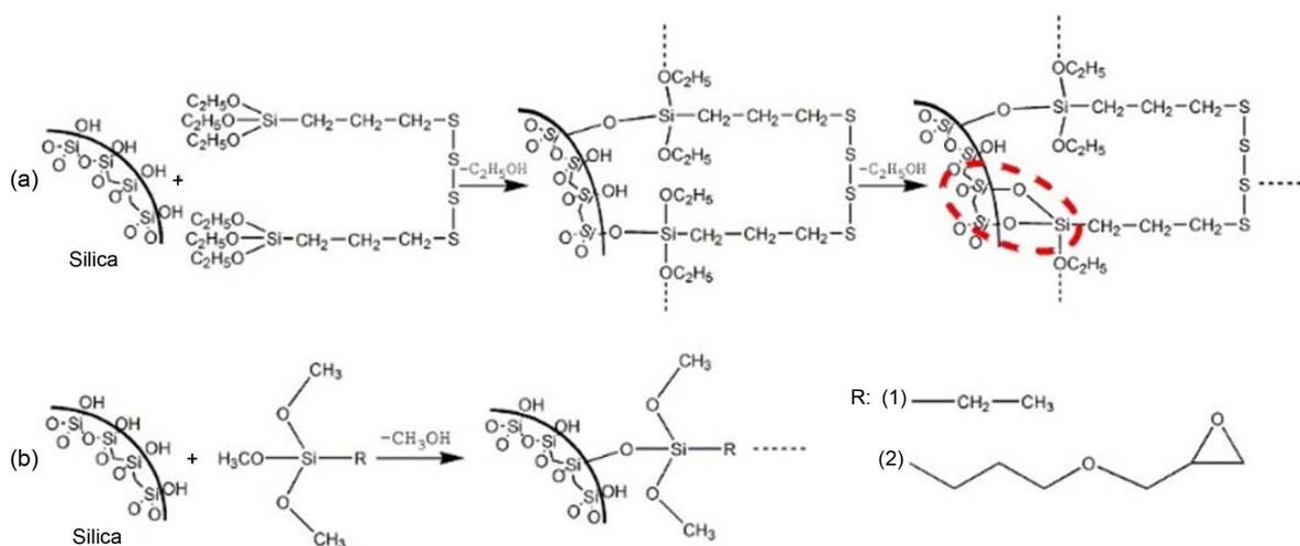
**Figure 10.** Proposed model of interactions between silica and silane coupling agents.
