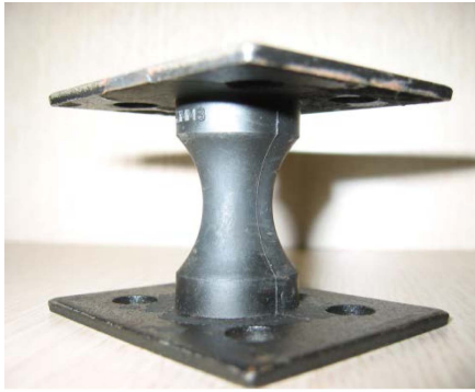
(a) 3 dimensional dumbbell specimen
