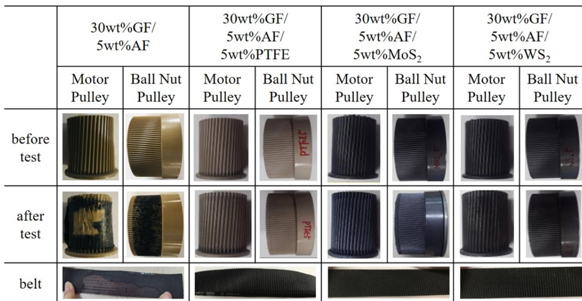
Figure 7. The comparative picture of motor and ball nut pulley after durability test. Each pulley was manufactured using the PPS composites containing different solid lubricant.
