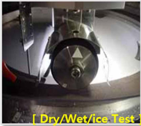
Figure 8. Friction tester for measuring rubber samples.
