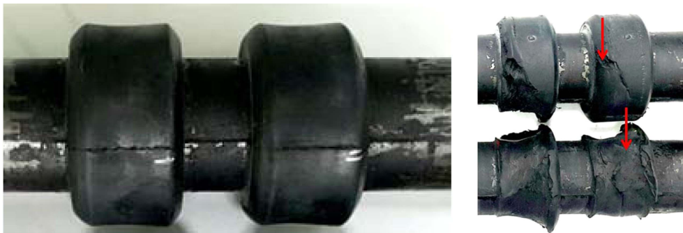
Figure 10. Fatigue failure of rubber bush.
