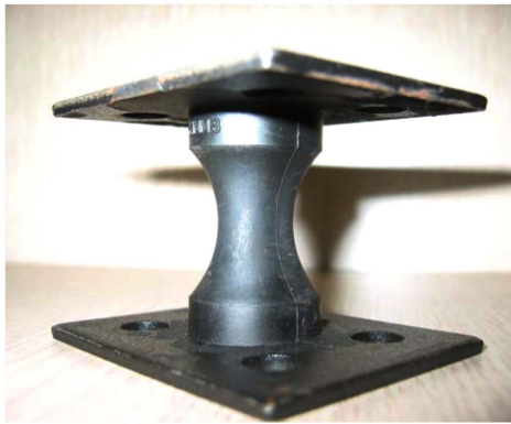
(a) 3-dimensional dumbbell specimen
