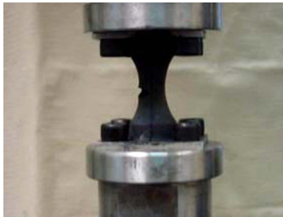
(b) Fatigue crack of 3-D dumbbell specimen
