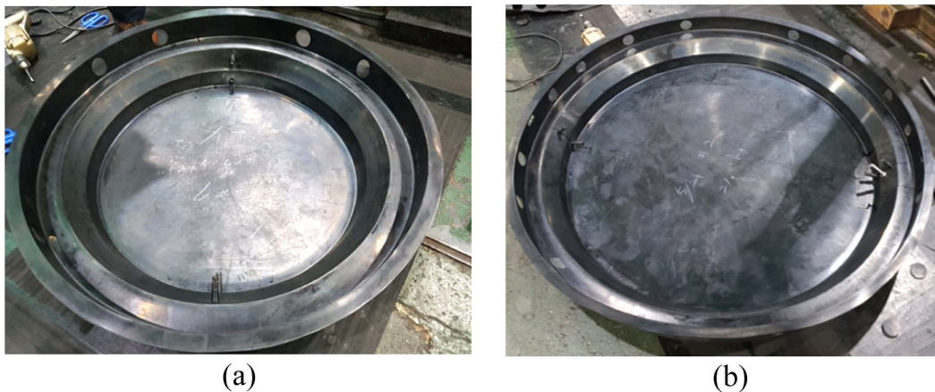
Figure 7. Diaphragm seal for nozzle dam: (a) 30 " diaphragm seal (b) 42 " diaphragm seal.
