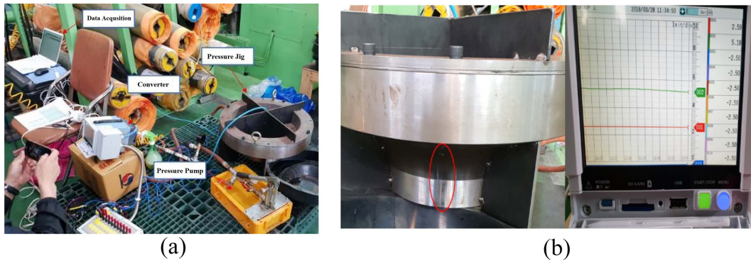
Figure 9. Performance test of diaphragm seal: (a) Performance test (b) Leakage test and result.
