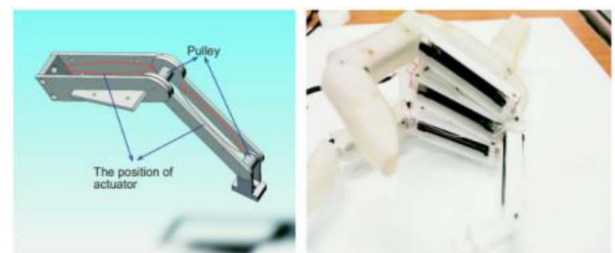
Figure 8. Multi-finger robotic hand with TSA. 31
