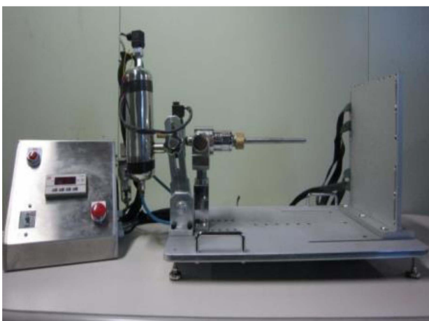
Figure 3. Low-velocity projectile test equipment and projectile.
