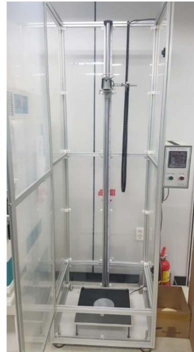
Figure 4. Ball drop impact test equipment.
