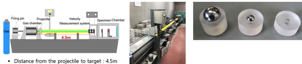
Figure 2. High-velocity impact test equipment and projectiles.
