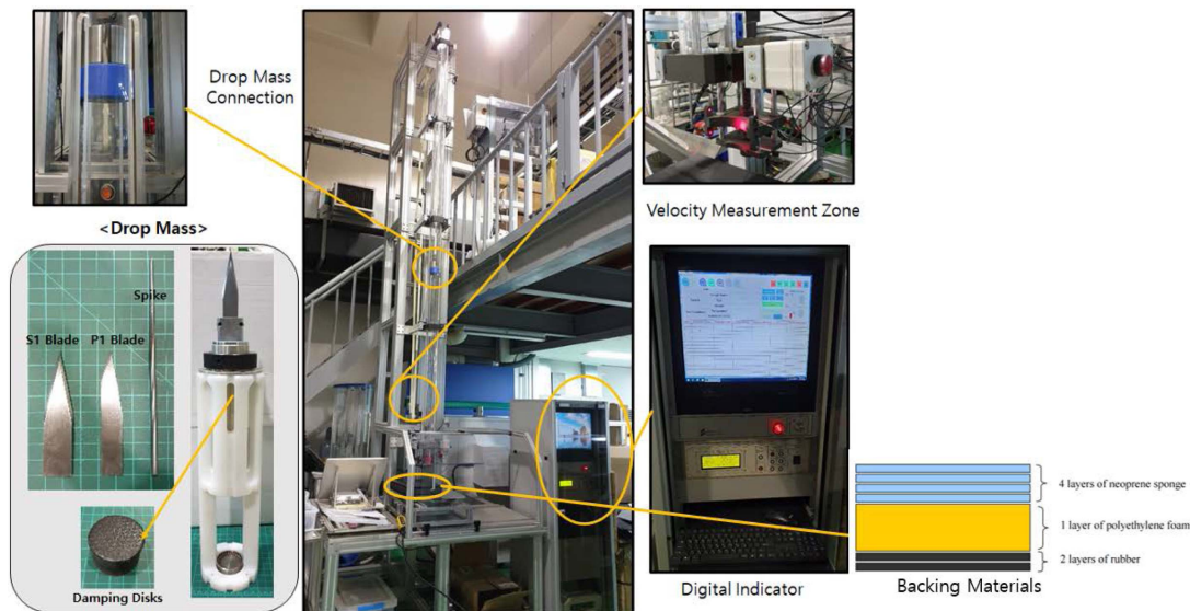
Figure 3. Test equipment of stab resistance test.
