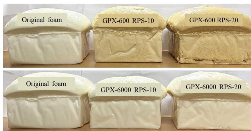
Figure 6. RPUFs based on different recycled polyol solutions obtained via glycolysis.
