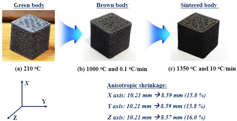
Figure 8. Anisotropic shrinkage in 3D printing structure after sintering, (a) 3D printed, (b) debound, and (c) sintered sample.
