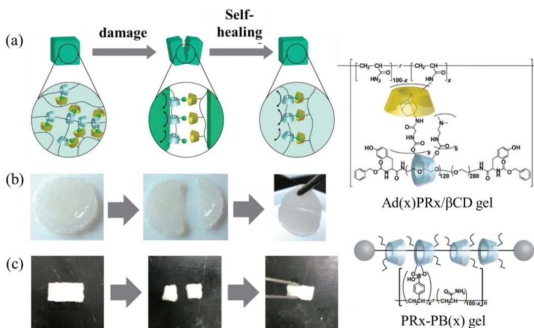
Figure 4. (a) Schematic illustration of self-healing of polyrotaxane gels and photographs showing self-healing behaviors of (b) polyrotaxane/β-CD and (c) polyrotaxane/phenylboronic acid gels. Reprinted from [14] with permission from The Chemical Society of Japan and [15] from Elsevier.
