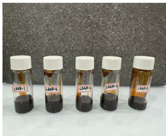
Figure 1. Synthesized epoxidized natural rubbers LENR-1–5.
