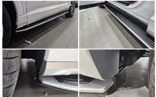
Figure 9. Side-Step installed in SUV for Vehicle TEST.
