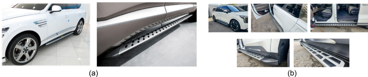
Figure 2. (a) Side-Step installed in SUV, (b) Side-Step installed in MPV.
