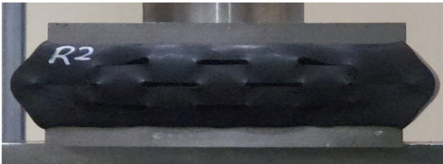
Figure 9. Static load test of the reference prototype of the passive shock isolator.
