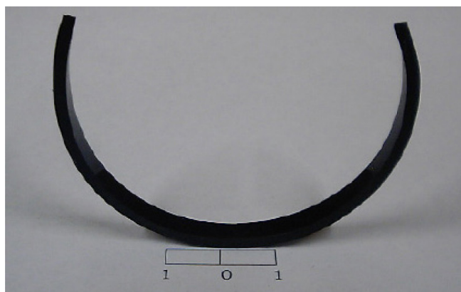
Figure 4. Picture of the deformed rubber sample after release following thermal aging under circular deformation.
